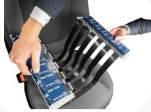
The amplifiers do not need to be removed from the frames.
